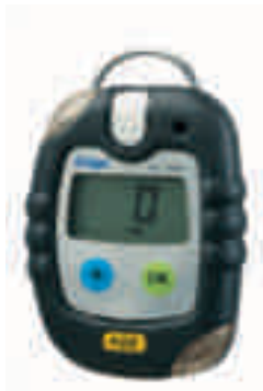
Dräger Pac 5000: Large concentration display.
