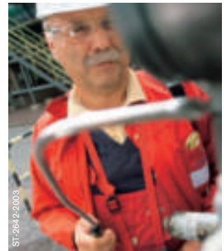
Dräger X-am 7000: Leaksearch made easy by generating audible clicks.
